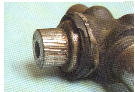
Figure 2-3 Brinelling of the trunnion
