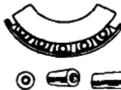
CRACKED INNER RACE
